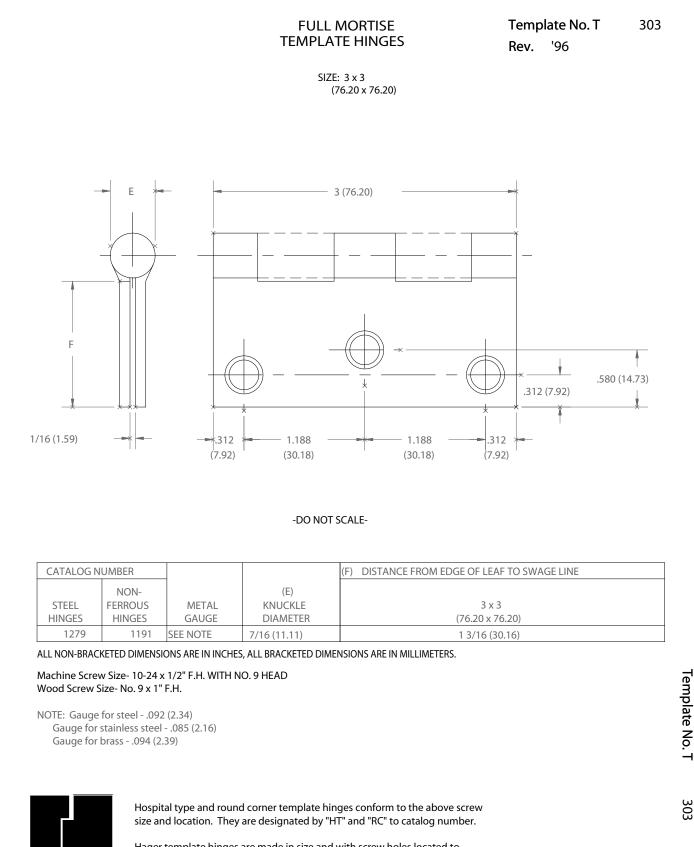
Hager template hinges are made in size and with screw holes located to conform to ANSI-A156.7.
